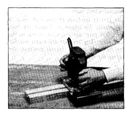
To install the straight guide, insert the guide bars into the holes in the tool base. Adjust the distance between the bit and the straight guide. At the desired distance, tighten the wing bolts to secure the straight guide in place.
